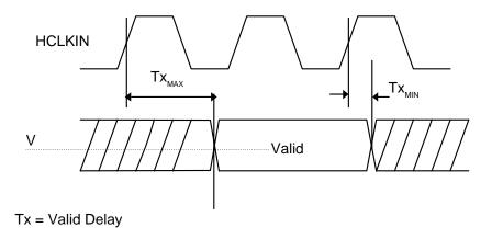
Figure 11: Valid Delay Timing
