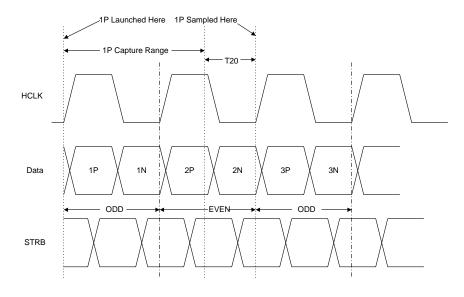
Figure 9: Source Synchronous Data Transfer
