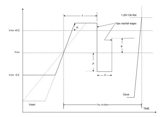
Figure 12: Standard Input Lo-to-Hi Waveform for Characterizing Receiver Ringback Tolerance
