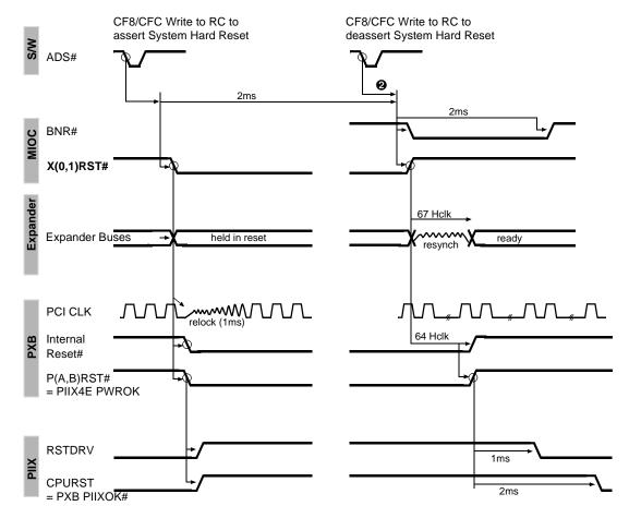
Figure 11-6: Software-Initiated PXB Reset
