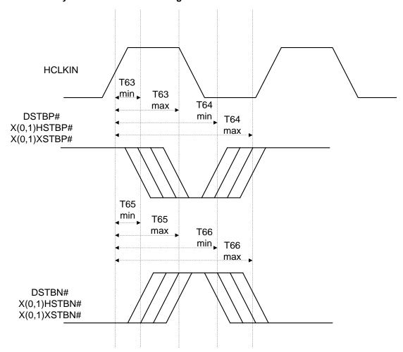
Figure 7: Source Synchronous Strobe Timing
