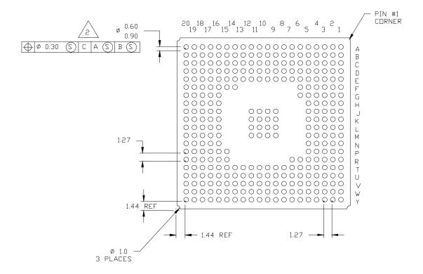
Figure 16: 324 BGA Dimensions Bottom View
