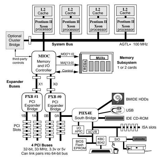
Figure 1-1: Simplified Intel® 450NX PCIset System Block Diagram
