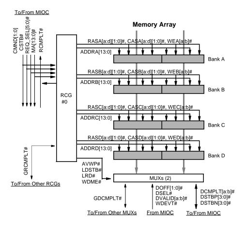
Figure 6-2: Example Showing RCG/MUX Control Signals
