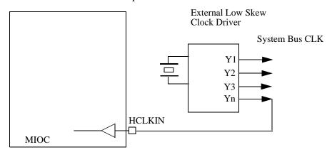
Figure 11-1: Host Clock Generation and Distribution
