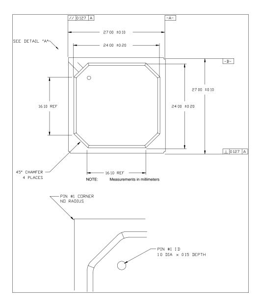
Figure 15: 324 BGA Dimension Top View
