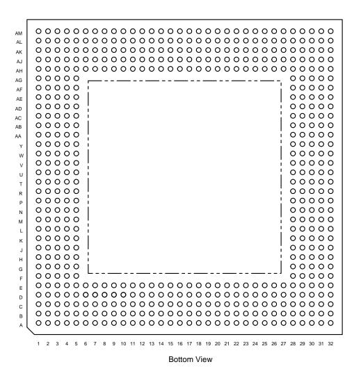
Figure 17: 540 PBGA pin grid
