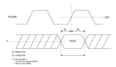
Figure 10: Setup and Hold Timings
