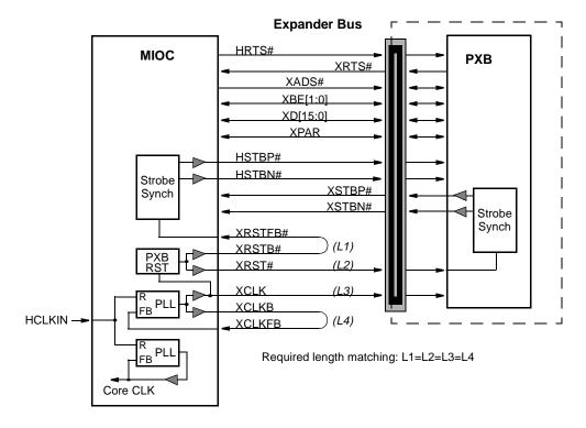
Figure 5-1: Expander Bus Clock Distribution
