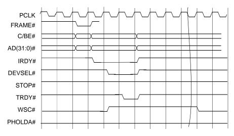
Figure 8-3: WSC# Signal Functionality
