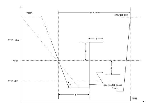
Figure 13: Standard Input Hi-to-Lo Waveform for Characterizing Receiver Ringback Tolerance
