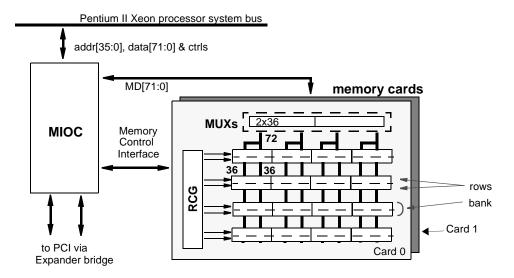
Figure 6-1: Memory Configuration using 2 Cards
