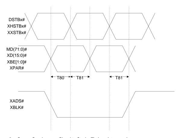
Figure 8: Source Synchronous Signal to Strobe Timings (at source)
