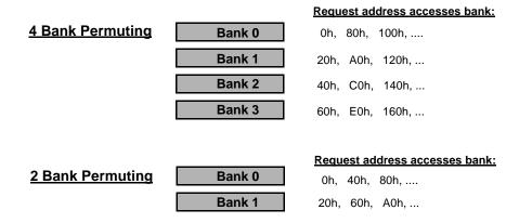
Figure 6-4: Effect of Address Bit Permuting on Bank Access Order
