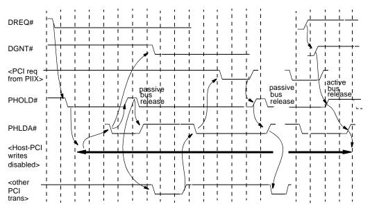
Figure 8-2: PHOLD#/PHLDA# protocol showing active and passive bus release
