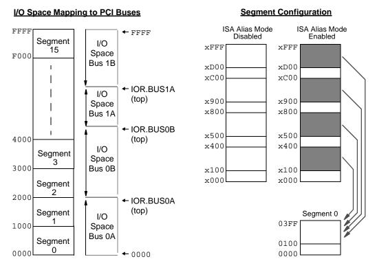
Figure 4-3: I/O Space Address Mapping
